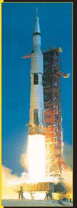
Apollo 11 roars toward the Moon. At launch, a rocket's engines must produce enough force and acceleration to overcome the pull of Earth's gravity. A rocket's liftoff is an illustration of Newton's third law: For every action there is an equal and opposite reaction.
